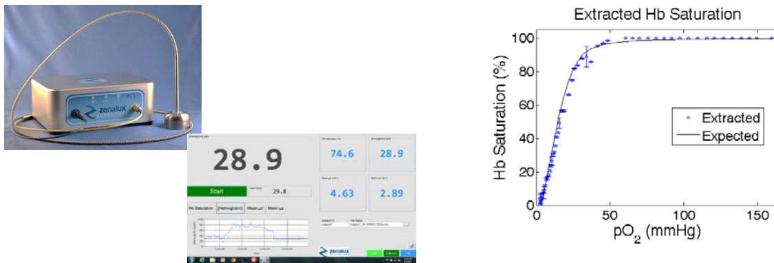
Figure 1: The Zenascope system, software output and an example measurement demonstrating the capability of the Zenascope. In the demonstration, hemoglobin saturation (the percentage of oxygenated hemoglobin relative to total hemoglobin content) measured by Zenascope was compared to oxygen pressure ( pO_2 ) measured by an invasive technique while oxygen was controllably depleted.
