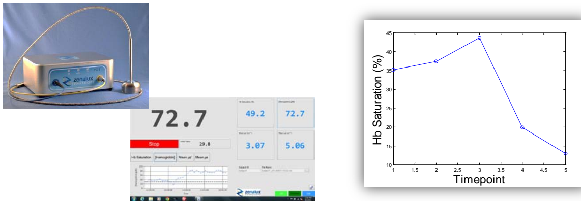
Figure 1: The Zenascope system, software output and an example measurement in which extracted hemoglobin saturation (the percentage of oxygenated hemoglobin to total hemoglobin content) was monitored in a subject at various time points during a 24 hour period.
